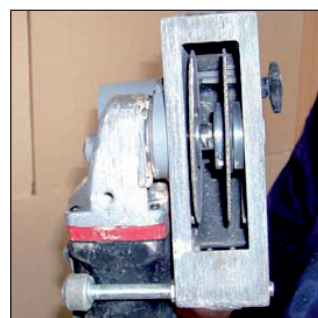
Special wall chaser with two diamond cutting blades and adjustable cut width and depth.
