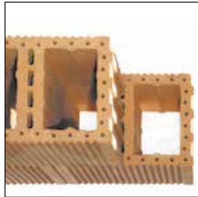
Offset in the wall bond, the channels are exactly on top of each other. This is important for floor-to-ceiling concrete backfill!
