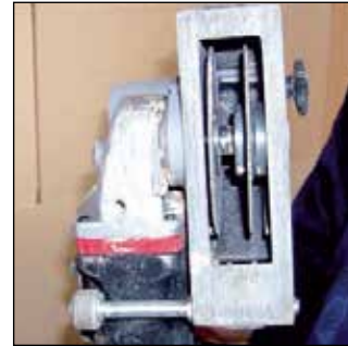
Special slot cutter with two diamond cutting discs and adjustable cutting width and depth.
