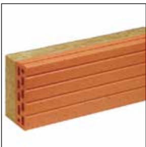
Slab edge shell with factory-glued insulation, a special hydrophobic mineral wool (WLG: 035), against formwork pressure.
