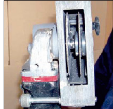
Special wall chaser with two diamond cutting blades and adjustable cut width and depth
